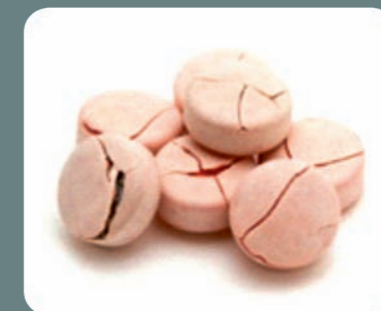
Example of Bad Tablet Coating
